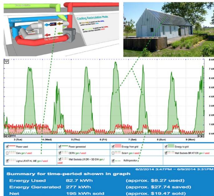
Data collected from the Gable Home over a seven-day period at the beginning of June 2014 is illustrated in figure 6 (See Figure 6). The week of June 3<sup>rd</sup> to 9<sup>th</sup> was hot and sunny with exterior
